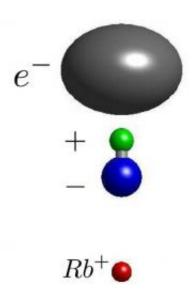
A schematic drawing of a new type of molecule with relatively gigantic dimensions, designed in theory by CfA scientists. The new molecule could be made in ultra-cold situations when a normal molecule is bound to an atom in a large excited state, for example as shown here with potassium-rubidium (KRb; the blue and green spots) joined to an excited large atom of rubidium (the red spot and gray electron cloud). Credit: S. Rittenhouse and H. Sadeghpour
