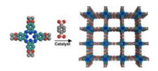
The Dichtel group in the Department of Chemistry and Chemical Biology has developed a method to organize organic dyes into stacked, porous two-dimensional sheets. These materials may ultimately be incorporated into inexpensive, flexible solar cells.
