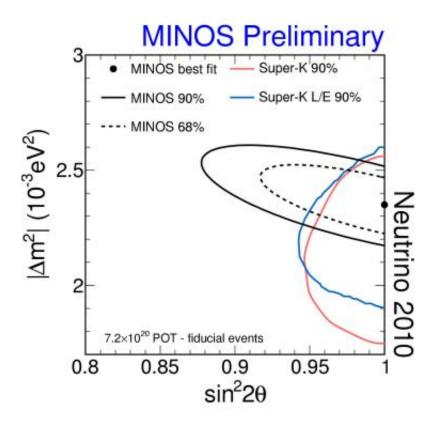
Neutrino oscillations depend on two parameters: the square of the neutrino mass difference,  $\Delta m2$ , and the mixing angle,  $\sin 22\theta$ . MINOS results (shown in black), accumulated since 2005, yield the most precise known value of  $\Delta m2$ , namely  $\Delta m2 = 0.0024 \pm 0.0001$  eV2.
