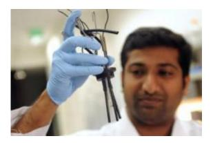
Dr. Prathap Parameswaran showing the electrode used in the microbial electrochemical cell (MEC). When the bacteria are grown in an oxygen-free, or anaerobic environment, they attach to the MXC's anode, forming a sticky matrix of sugar and protein. This living matrix, known as the biofilm anode, is a strong conductor. Credit: The Biodesign Institute at Arizona State University
