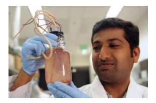
Microbial electrochemical cells or MXCs are able to use bacterial respiration as a means of liberating electrons, which can be used to generate current and make clean electricity. MXCs resemble a battery, with a Mason jar-sized chamber setup for each terminal. The bacteria are grown in the "positive" chamber (called the anode). Credit: The Biodesign Institute at Arizona State University
