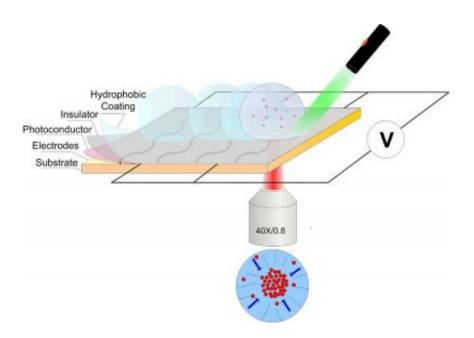
This diagram depicts the design of a new "hybrid optoelectric" device. The device uses a tightly focused infrared laser beam to position tiny particles, such as viruses and bacteria, onto a sensor. (Han-Sheng Chuang/Purdue University Birck Nanotechnology Center)
