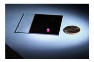
This image shows a new "hybrid optoelectric" device, developed by researchers at Purdue. The device uses a combination of light and electric fields to position droplets and tiny particles, such as bacteria, viruses and DNA, representing a potential new tool for medical diagnostics and crime-scene testing. Credit: Craig Snoeyink/Purdue University Birck Nanotechnology Center
