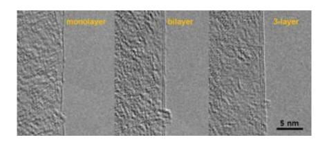
High-resolution TEM images showing the folded edges of as-grown graphene films with different number of layers. Image credit: Nature Nanotechnology (doi:10.1038/nnano.2010.132)
