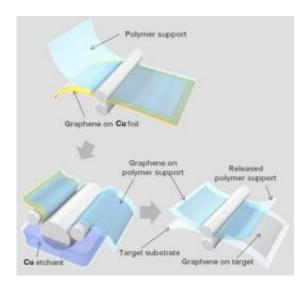
The researchers built up a graphene layer on copper foil and then used rollers to transfer the graphene to a polymer support and then onto a final substrate. Image credit: Nature Nanotechnology. (doi:10.1038/nnano.2010.132)
