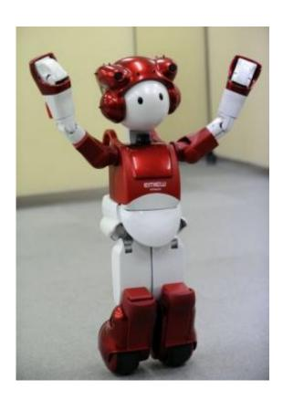
A picture shows Japan's electronics giant Hitachi's humanoid robot "Emiew2", 80cm tall and weighing 14kg, which can move over uneven ground and small gaps on its wheeled legs at the company's laboratory in Tokyo. The robot is also equipped with 14 microphones on its helmet which can pick out human voices from background noise.
