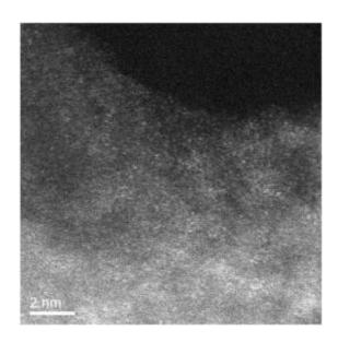
Aberration corrected STEM image of Pd/ZnO treated in flowing H2 at 500°C. The bright spots represent single atoms of Pd dispersed on the ZnO surface (image obtained by L. F. Allard at ORNL)
