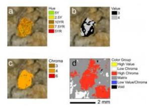
These are digital images of soil features classified by hue, value (lightness or darkness) and chroma (saturation). Computer-assisted classification of soil types can be a more robust alternative to comparing samples in the field with printed color charts. Credit: Courtesy Kevin O'Donnell, University of Missouri
