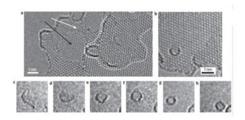
These images from a transmission electron microscope show the formation of fullerene from graphene. In (a), the edges of the graphene sheet continuously change shape when exposed to the e-beam. (b) shows the final product, while (c)-(h) show close-ups of the sequence of a graphene flake transforming into a fullerene. Image credit: Andrey Chuvilin, et al.
