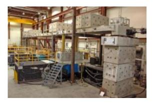
The 200-ton, four-span bridge was built over several months atop the 14-foot square shake tables at the world-renowned University of Nevada, Reno large-structures lab. The innovative bridge was hit with nine increasingly more powerful earthquakes over several days, and survived, giving researchers reams of data collected from sensors through 350 channels. Credit: Photo by Mike Wolterbeek, University of Nevada, Reno
