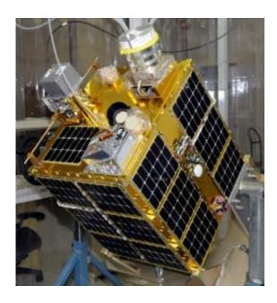
FASTSAT is a small, microsatellite class spacecraft bus that will carry six experiment payloads to low-Earth orbit. One of FASTSAT's mission objectives is to demonstrate its ability to eject a nanosatellite from a microsatellite while avoiding re-contact with the FASTSAT satellite bus. Credit: NASA/MSFC, Doug Stoffer
