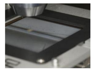
This photograph shows microshutters being examined with a microscope. A hair is visible in the picture for size comparison. Credit: NASA/Chris Gunn
