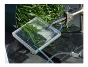
Cheatgrass photosynthesizes in an artificial atmosphere during a labeling experiment. The experimental "chamber" is essentially a CD jewel case fitted with an O-ring. Credit: Jacob Schaefer
