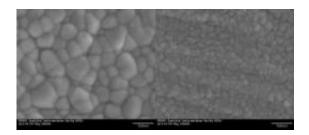
By applying a 60 Hertz alternating current field, researchers were able to reduce the grain size of ceramics by 63 percent -- and eliminated porosity at 1,250 degrees Celsius, as opposed to the 1,500 degrees Celsius needed without the electric field. Credit: Dr. Hans Conrad, North Carolina State University
