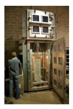
Honeybee Project Engineer Gale Paulsen adjusts settings for the Mars Simulation Chamber in preparation for a test of the company's rotary-sonic drill. Credit: Henry Bortman
