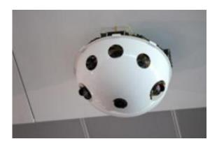
ISIS takes new video-camera and image-stitching technology and bolts it to a ceiling, mounts it on a roof, or fastens it to a truck-mounted telescoping mast. Credit: DHS S&T
