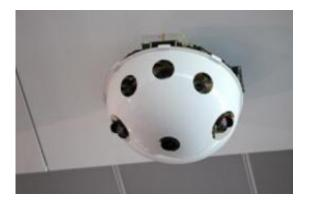
ISIS takes new video-camera and image-stitching technology and bolts it to a ceiling, mounts it on a roof, or fastens it to a truck-mounted telescoping mast. Credit: DHS S&T
