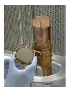
Each CDMS detector is a 230-gram germanium crystal. Six detectors are stacked to form one of the five towers that make up the whole apparatus.
