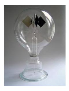
Pictured above is a Crookes radiometer -- also known as the light mill -- which consists of an airtight glass bulb, containing a partial vacuum. Inside are a set of vanes which are mounted on a spindle. The vanes rotate when exposed to light, with faster rotation for more intense light, providing a quantitative measurement of electromagnetic radiation intensity.
