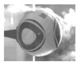
One of the main differences among soccer balls is how much the air flow follows the ball's surface. Turbulent air flow would hug the curvature of the ball, reducing drag. In this high-speed video of the Jabulani ball, however, Caltech scientists demonstrate that the air flow actually separates after about halfway across the ball.
