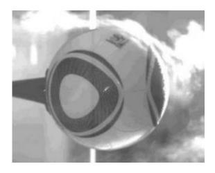
One of the main differences among soccer balls is how much the air flow follows the ball's surface. Turbulent air flow would hug the curvature of the ball, reducing drag. In this high-speed video of the Jabulani ball, however, Caltech scientists demonstrate that the air flow actually separates after about halfway across the ball.
