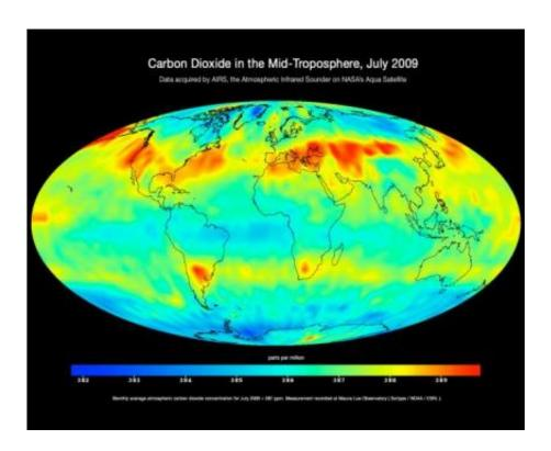
Data from the Atmospheric Infrared Sounder instrument on NASA's Aqua satellite shows large-scale patterns of carbon dioxide concentrations that are transported around Earth by the general circulation of the atmosphere. Credit: NASA/JPL
