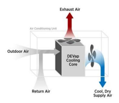
This illustration shows how the DEVap cooling core uses water and liquid desiccant to draw in outside air, exhaust some of that air and return cool, dry air to the area being cooled. DEVap's integrated evaporative component and its desiccant drying process offer improved dehumidification and, thus lower costs and much lower energy usage.
