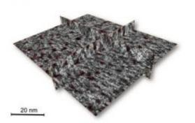
An image showing nanoscale pores in the dielectric material. (Huolin Xin/Muller Group)
