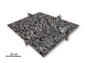
An image showing nanoscale pores in the dielectric material. (Huolin Xin/Muller Group)
