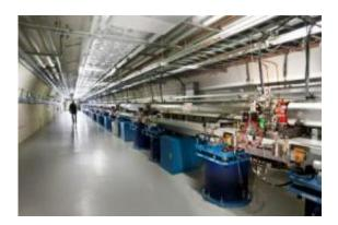
SLAC National Accelerator Laboratory's LCLS-II will occupy the second (left) half of the subterranean Undulator Hall, which was designed to accommodate a pair undulator arrays operating in tandem. The undulator array for LCLS-I, seen here, began generating pulses of X-Ray laser light in April 2009. Credit: Image courtesy of Brad Plummer/SLAC
