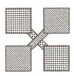
This illustration shows the two test mass assemblies, which consists of two pairs of aluminum cubes. Four tracking frequency laser gauges measure each cube's acceleration as it falls to Earth from altitudes of up to 1200 km. Image credit: Reasenberg and Phillips.
