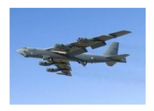
In this image provided by the U.S. Air Foce an X-51A Waverider rides under the wing of a B-52 Stratofortress Dec. 9, 2008. A similar X-51A successfully launched from a B-52 Stratofortress, Wednesday May 26, 2010. The Rocketdyne-built air breathing scramjet engine accelerated the vehicle to Mach 6. It was the longest supersonic combustion ramjet-powered hypersonic flight to date. (AP Photo/US Air Force - Mike Cassidy)
