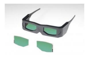
Toshiba Mobile Display has developed an OCB (Optically Compensated Bend) liquid crystal display panel for 3D glasses suitable for watching 3D television, enjoying 3D movies, or playing 3D games.
