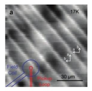
A probe measuring the penetration depth of a magnetic field into a hightemperature superconductor reveals stripes that hint at a connection between crystal boundaries and superconductor quality. Credit: B. Kalisky, J.R. Kirtley, J.G. Analytis, Jiun-Haw Chu, A. Vailionis1, I.R. Fisher and K.A. Moler
