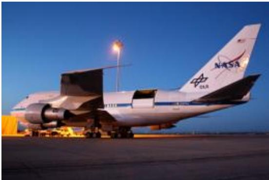
The Boeing 747SP used for the SOFIA project is 45 feet shorter than a modern 747, making it lighter and more able to make long transoceanic flights without stopping to refuel.
