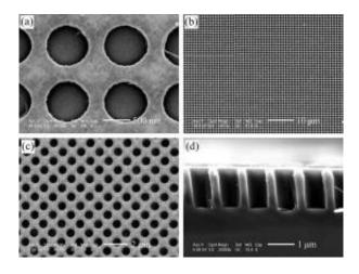
These scanning electron microscope images show the silicon nanoholes at different scales, and (d) shows a cross-sectional view. Image credit: Peng, et al. ©2010 American Chemical Society.
