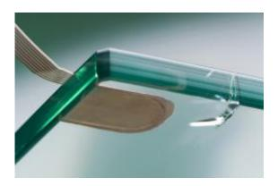
The sensor is located on the rim of the sheet of glass. It is linked to the building control systems by cable. (© K. Dobberke/Fraunhofer ISC)
