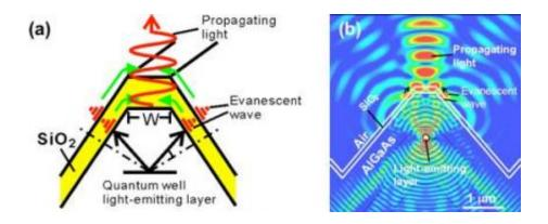
The illustration in (a) shows evanescent waves coupling at two interfaces on the flat planes of a ridge. Figure (b) shows the simulated electromagnetic field intensity of the structure. Image credit: AIST.
