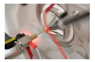
Ionization of the sample with electro spray prior to the mass spectrometer measurement. Image: Axel Griesch
