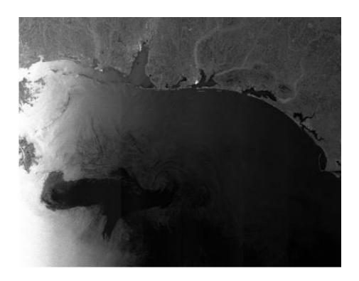
In this image, acquired by Envisat's Advanced Synthetic Aperture Radar instrument on 28 April 2010 at 03:45 UTC, the oil spill is visible as a lighter grey whirl on the left side of the large black pattern stretching across the Gulf. Credits: ESA
