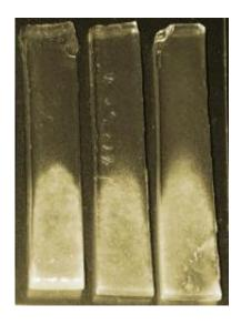
Experimental hydrogel scaffolds prepared at NIST for culturing bone cells clearly show the dependence of bone mineralization on the stiffness of the gel. Deposited minerals are denser at the bottoms of the gradient gels, which are progressively stiffer from top to bottom. Strips are approximately 1 x 6 cm. (Color added for emphasis.) Credit: Chatterjee, NIST
