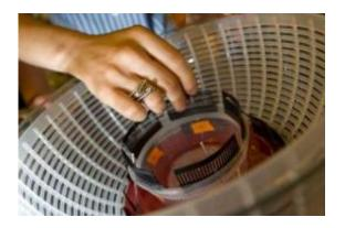
A simple salad spinner is the basis for a centrifuge that can be used to separate blood in resource-poor settings easy without access to electricity. Credit: Jeff Fitlow/Rice University
