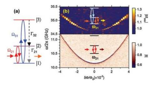
Quantum amplification by an artificial atom. Part (a) shows a sketch of a threelevel artificial atom in which population inversion can be created by pumping the atom from the ground state to the second excited state. Part (b) shows the spectroscopy of the three-level atom.
