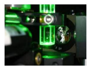
A 5-micrometer glass bead levitated in air by a single laser beam from below. This optical trap is formed by the balance between the scattering force from the laser beam and the gravitational force on the bead. Tongcang Li, et. al. used a similar optical trap to study the Brownian motion of a trapped bead in air with ultra-high resolution. Their paper is published in Science. Credit: Tongcang Li, the University of Texas at Austin
