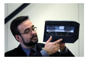
This car speedometer cover with two anti-reflective circular surface areas was manufactured in just one step. (© Fraunhofer IWM)
