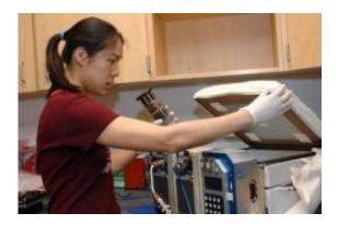
CU-Boulder aerospace engineering sciences graduate student Christine Fanchiang shown with BioServe Space Technologies hardware, including a Commercial Generic Bioprocessing Apparatus and a cylindrical, fluid-processing device known as a GAP that will be used for microorganism experiments in low gravity aboard the final flight of Atlantis. (Photo by Patrick Campbell/University of Colorado)
