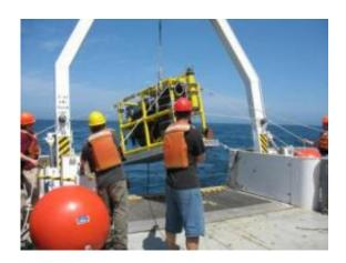
NRL scientists and R/V Cape Hatteras crew deploy the Deep Towed Acoustics Geophysics System (DTAGS) after it is outfitted with an aluminum landing plate that couples the sound energy generated by DTAGS directly into the seafloor. The large orange sphere is one of the floats used in the seafloor-mounted vertical hydrophone arrays, which listened to the sounds generated by DTAGS and their echoes off the seafloor. Credit: Naval Research Laboratory
