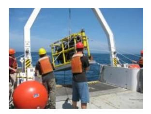
NRL scientists and R/V Cape Hatteras crew deploy the Deep Towed Acoustics Geophysics System (DTAGS) after it is outfitted with an aluminum landing plate that couples the sound energy generated by DTAGS directly into the seafloor. The large orange sphere is one of the floats used in the seafloor-mounted vertical hydrophone arrays, which listened to the sounds generated by DTAGS and their echoes off the seafloor. Credit: Naval Research Laboratory
