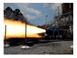
(PhysOrg.com) -- Fire and sparks flew as a 24-inch-diameter solid rocket motor was successfully tested May 27 at NASA's Marshall Space Flight Center in Huntsville, Ala. The 21-second firing tested a NASA sub-scale motor designed as a versatile, quick-turnaround and low-cost way to determine the performance of new materials and designs.
