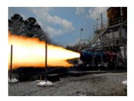
(PhysOrg.com) -- Fire and sparks flew as a 24-inch-diameter solid rocket motor was successfully tested May 27 at NASA's Marshall Space Flight Center in Huntsville, Ala. The 21-second firing tested a NASA sub-scale motor designed as a versatile, quick-turnaround and low-cost way to determine the performance of new materials and designs.
