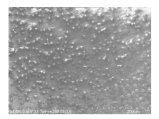
Fibroblasts growing on titanium alloy coated with nanotubes
