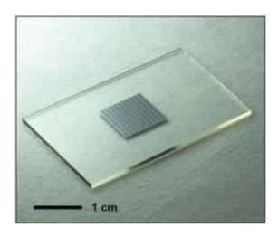
Image of a printed GaAs solar cell with a size ~10 x 10 mm2 on a glass substrate, with simple, metal grid contacts. Image copyright: Nature, DOI:doi:10.1038/nature09054
