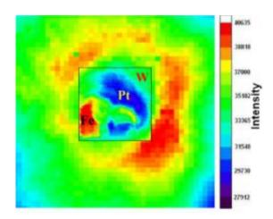
Measurement of x-ray transmission (red highest, blue lowest) through a mixture of iron, platinum, and tungsten compressed to 282 GPa. The outer image, 40  $\mu$ m x 40  $\mu$ m, is resolved into 1- $\mu$ m pixels, and shows only the roughly circular boundary of the diamond face compressing the sample. The inner portion, 15  $\mu$ m x 15  $\mu$ m, is resolved into 250-nm pixels, and clearly shows distinct regions of the three metals.
