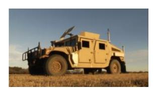
This military HUMVEE is outfitted with Southwest Research Institute's AVM-375 low-profile antenna set, which consists of four specially designed antenna arrays distributed around the body of the vehicle to reduce the system's visible signature. The antenna set, shown in lighter-colored packaging, improves mission stealth and vehicle mobility while providing geolocation of enemy forces from a single moving platform.
