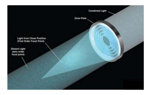
The alternating rings on zone plates bring faraway and nearby objects into focus simultaneously.
