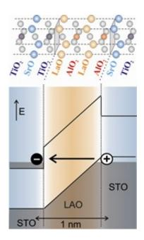
In a stacked atomic structure of lanthanum oxide with a strontium titanate capping layer on a substrate of strontium titanate (crystal structure from left to right, top of illustration), the internal potential in the LAO layer brings about a redivision of charge. The resulting electrons on the interface leave behind holes that are just one nanometre apart. The electrons (left) and gaps (right) in parallel produce a contribution to the electrical conductivity.
