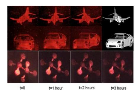
These digital camera images show holograms created with the photorefractive polymer in an updatable holographic 3D display. Image credit: Christenson, et al. ©2010 IEEE.
