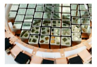
Light sensors making up the lower detector on the XENON experiment. Image credit: Guillaume Plante
